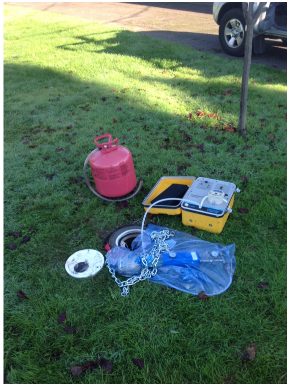
Photograph 14. Soil gas sampling setup, November 2012.
