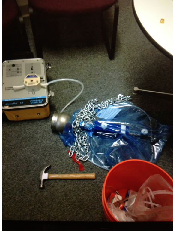
Photograph 19. Subslab sampling setup, November 2012.
