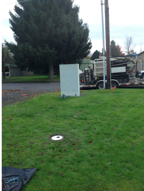
Photograph 11. Installed soil gas sampling port outside the Fire Station, November 2012.
