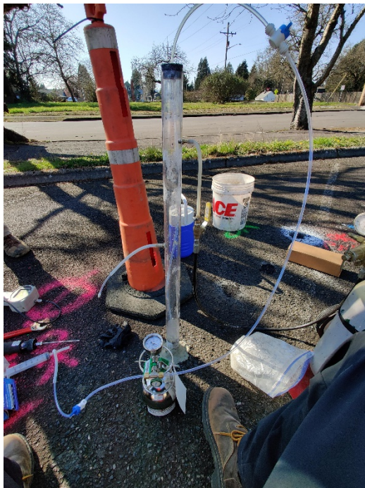
Photo 2. Boring SB-2 – picture of the shroud setup for collecting the soil-gas sample. Photo taken facing west.
