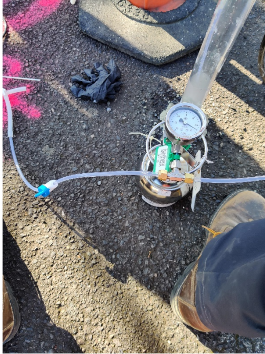
Photo 1. Boring SB-2 – collecting the soil-gas sample. Photo taken facing west.
